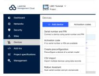
In the next window, enter the serial number and Cloud PIN of the device. Then confirm with the button **Add new device**.
