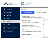
Create an activation code by following the instructions in the dialog. This activation code allows you to integrate the LANCOM device into this project at a later time.
